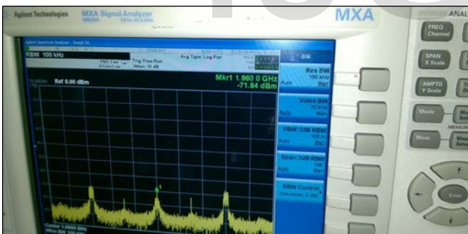
Fig. 8: MXA Signal Capture of the OFDMA Carriers
